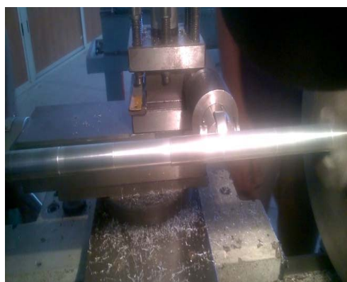
Fig. 6: Roller burnishing operation. Experimental Details
